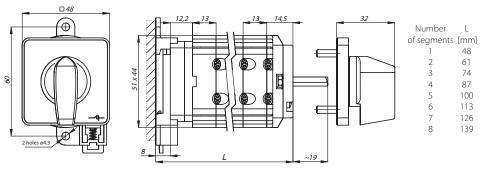
$<sup>^{*}</sup>$  It is possible to increase the length by a multiple of 13 mm
