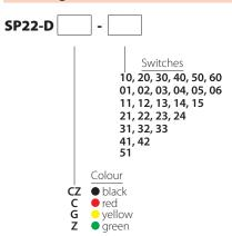
Description: the first digit represents the number of normally open circuits, the second digit represents the number of normally closed circuits.
