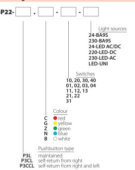
Description: the first digit represents the number of normally open circuits, the second digit represents the number of normally closed circuits.
