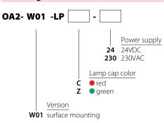
OA2-W01-LPC-230 Red lamp  ${\bf 230V}$  in a housing with a glass cover - OA2-W01-LPZ-24 Green lamp  ${\bf 24V}$  in a housing with a glass cover -
